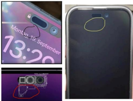
Behind the screen sensors minimize cutout but may distort screen
